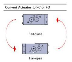
To convert from fail-safe open to close, or vice-versa, reattach the EPV to the EVA by rotating the EPV 180°. Switch orientation of grub screw to ensure non-interference with installation.
